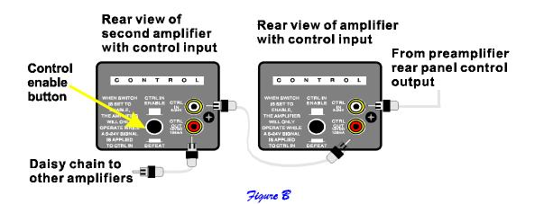
If the control function is desired, each unit in the system must remain connected at all times and the control must be enabled. To enable the control function, the CTRL ENABLE button must be out for each controllable amplifier in the system. For more information on the amplifiers output status under various control conditions, refer to the table below.
